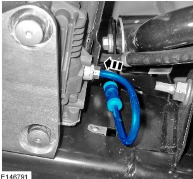
33. Connect the new air line link pipe.
