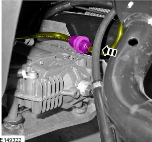
39. Install the suspension compressor lower cover.
