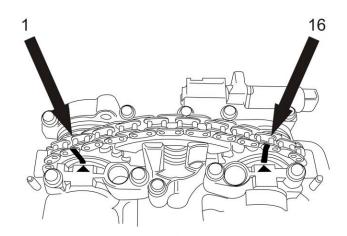
• Check that there are 16 rollers between the markings of the camshafts gears.
