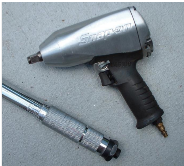
For lugs, nix on the 1/2-inch impact, and affirmative on the torque wrench.
